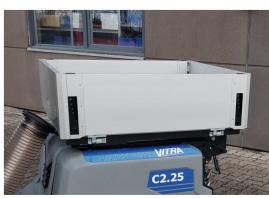
The truck bed is built as a strong steel/aluminium construction, which ensures low weight and large load capacity.
