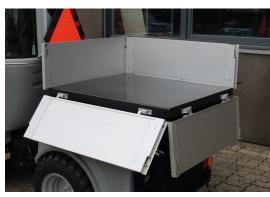
The truckbed is constructed with a completely flat bottom and fold-down aluminium sides and tailgate.
