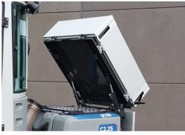
As an option, the truck bed can be mounted with hydraulic tilt for easy unloading - For example, directly in a rear-mounted spreader.
